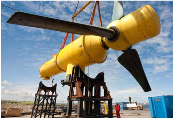
(a) The 500KW turbine on site at Hatston Quay, Orkney
