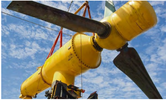
(a) The 500KW DEEPGEN III being lifted.
